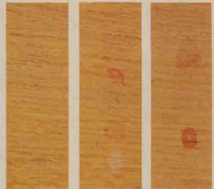
Aqua Zar Polyurethane ( left ) repelled our water-based stain completely, while Valspar Polyurethane ( center ) allowed some staining. General Finishes Polycrylic ( right ) stained deeply.
